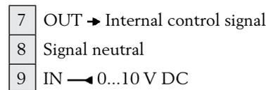
Terminals 7 and 9 are connected by a factory-mounted wire strap. Remove the wire strap when using external control signal.
